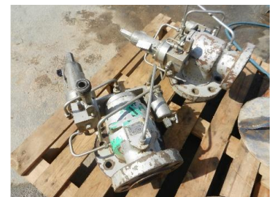
Pressure Safety Valve re-calibration.
