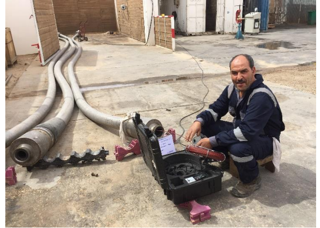
Camera inspection in HP hose.
