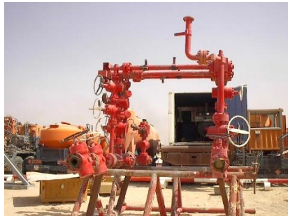
Manifold with integral spools and API valves.
