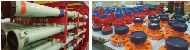
Temporary piping, adaptors, wing unions, clamp connectors.
